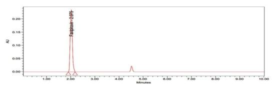
Figure 16: Purity Plot of Hydrolysis degradation
